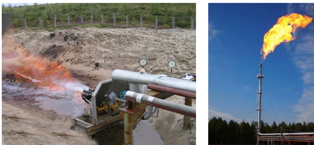
Figure 1. Horizontal and vertical arrangement flare stacks
