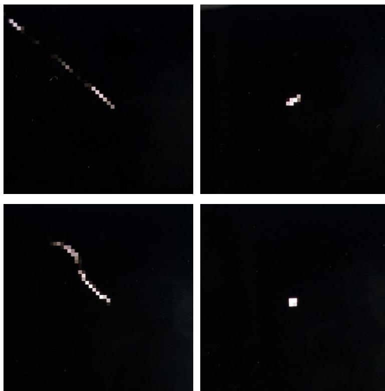
Figure 7. Recorded images by the CCD array of a cell phone showing the passage of a high-energy particle (Source: MUT)
