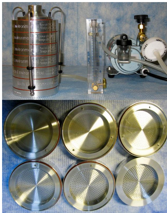
Figure 5. Six-stage Andersen cascade impactor type TE-10-800 (source: own research).
