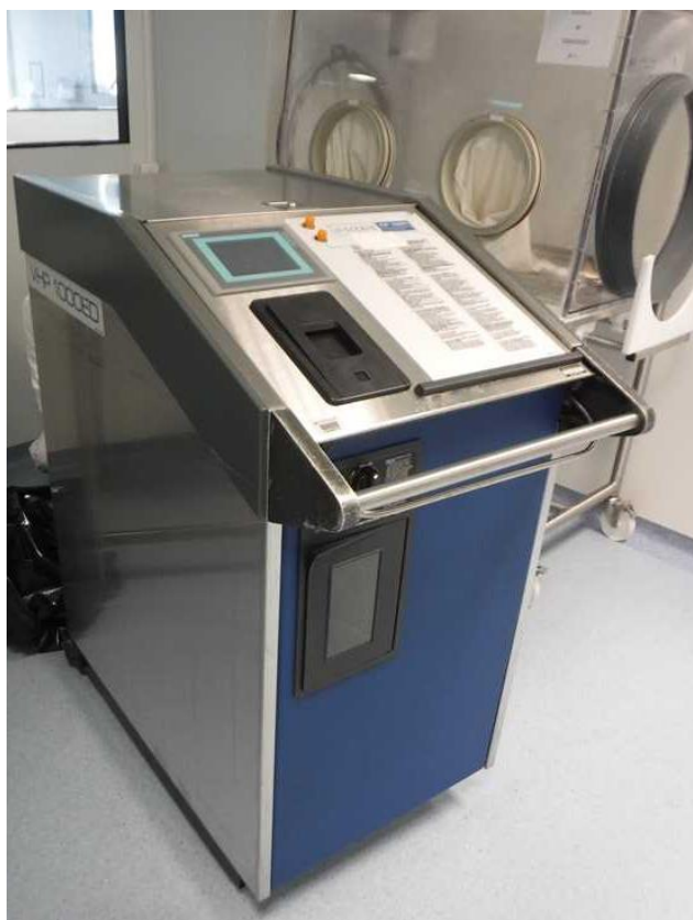
Figure 3. Steris VHP 1000 ED - EDS 230 Vaporised Hydrogen Peroxide Generator. (source: www.equipnet.com )
